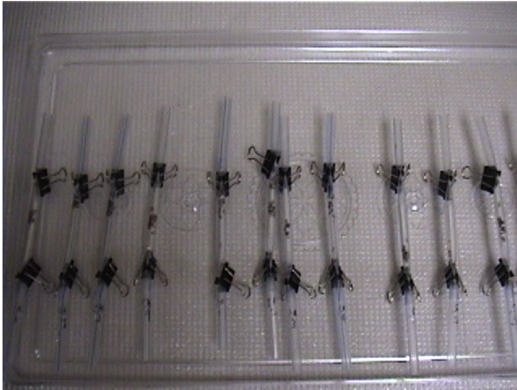
Figure 1. Visual of the “straw technique” described by Drees (2002) used to assess worker ant mortality to various dilutions of metaflumizone.
