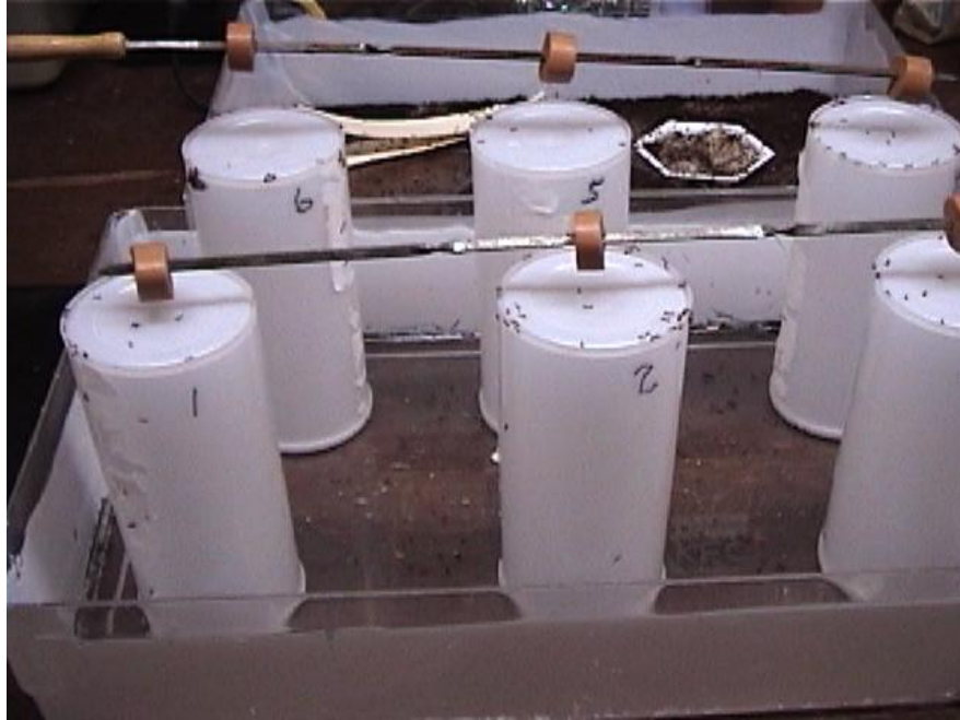
Figure 2. Apparatus used to assess foraging ant visual olfactory response to near presence of hot dog slice food lures with laboratory colony tray in background, foraging arena containing tall cylindrical plastic foraging towers in foreground and skewered hot dog slices positioned at various distances above foraging towers.
